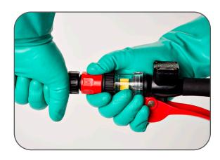
When filling operations are complete, turn the inverter off and store the red output hose.
