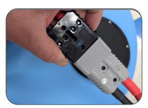
Connect SB175 from Inverter to the battery in the pallet rider truck.
