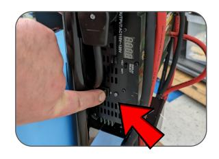
Turn the switch on to operate.
