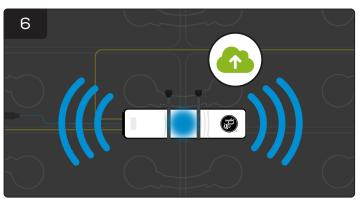
The radio is now enabled, and the blue LED remains illuminated until all data has been transmitted to eGO!CloudLink.
