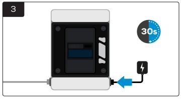
Connect the eGO!CloudLink with power connection. And wait for 30 seconds.
