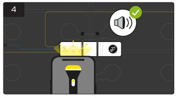
Take a bright flash light (\*A mobile phone flash light will be adequate) and place directly on top of the white circle on eGO!Pro until you hear a beep along with blue LED.
