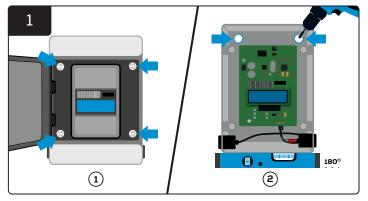
Open and unscrew the grey cover. Mount the control box to the wall using four screws/anchors and a level. Make sure it is firmly attached to the wall. Rescrew the cover.
