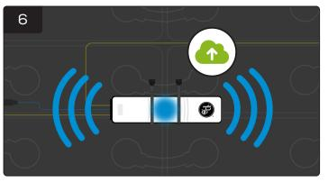
The radio is now enabled, and the blue LED remains illuminated until all data has been transmitted to eGO!CloudLink.
