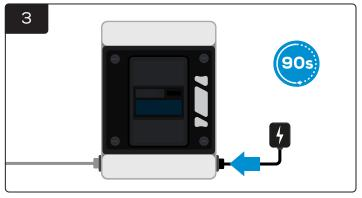
Connect the eGO!CloudLink with power connection. And wait for 90 seconds.
