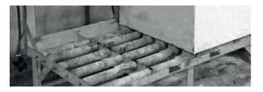
Traditional battery racking systems are all the same. They are a welded frame with some standard conveyor rollers.
