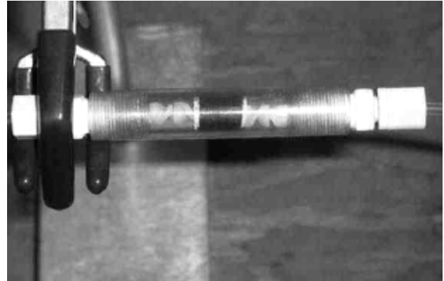
Figure 4: Packed Filter bed reactor used to determine the H 2 S absorption capacity/rate of PbO and PbO 2 .
